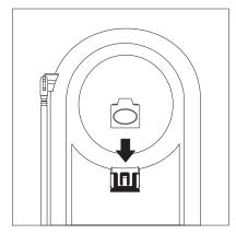
4. Push down on the Handset retainer until it snaps into place.
